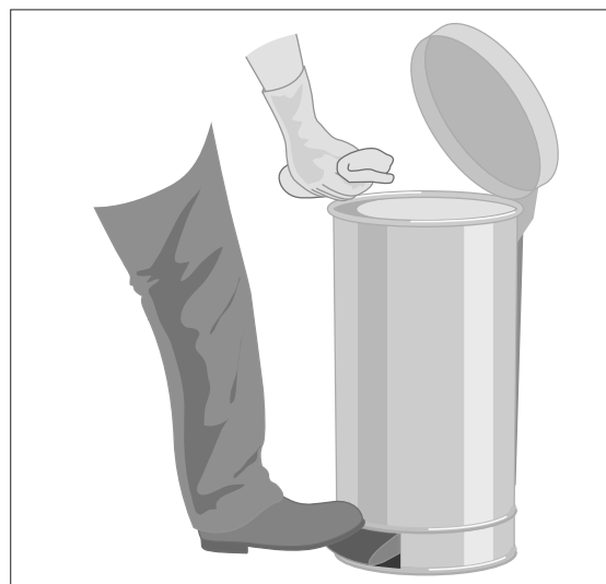
Figure 15: A fire-resisting pedal bin for rags
